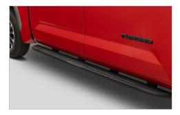
Not only do the Running Boards assist with entering your Tundra, they also help protect the lower body from road debris. Constructed from highly durable aluminum for corrosion-resistance, they feature a wide-step surface with rubber grommets to help ensure a secure footing. Engineered to mount securely to the Tundra's sides using existing mounting points.
