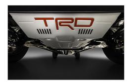
Enhances Tundra's tough, capable stance and helps protect vehicle underbody from damage that can result from flying stones, salt, branches, ice chunks, and other types of road debris. Made from stamped and formed 1/4-in.-thick silver powder-coated aluminum.
